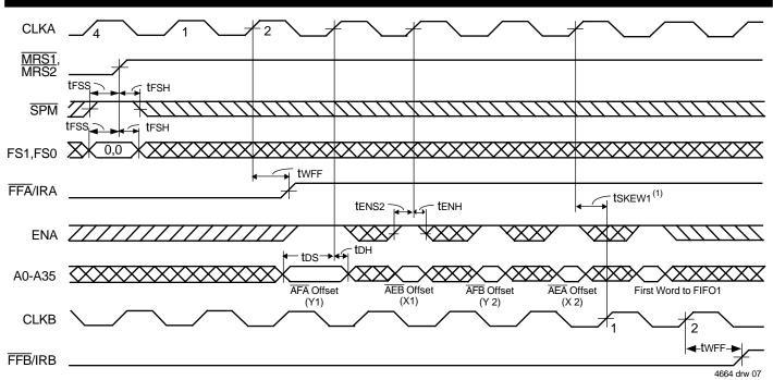
1. tskewi is the minimum time between the rising CLKA edge and a rising CLKB edge for FFB/IRB to transition HIGH in the next cycle. If the time between the rising edge of CLKA and rising edge of CLKB is less than tskewi, then FFB/IRB may transition HIGH one CLKB cycle later than shown.
