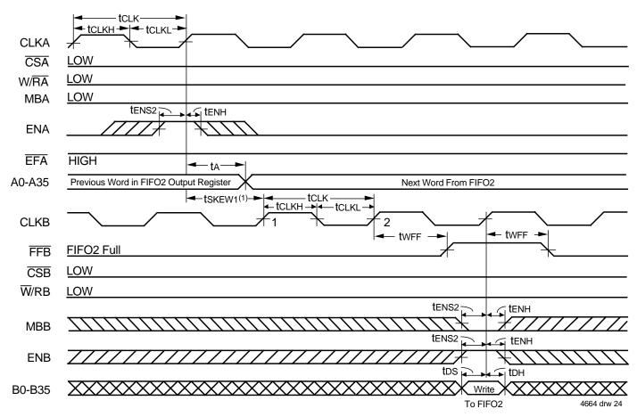
1. tskewi is the minimum time between a rising CLKA edge and a rising CLKB edge for FFB to transition HIGH in the next CLKB cycle. If the time between the rising CLKA edge and rising CLKB edge is less than tskewi, then FFB may transition HIGH one CLKB cycle later than shown.
