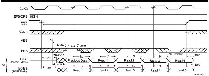
1. Unused bytes B9-B17, B18-B26, and B27-B35 are indeterminate for byte-size reads.
