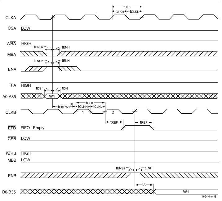
1. tskewi is the minimum time between a rising CLKA edge and a rising CLKB edge for EFB to transition HIGH in the next CLKB cycle. If the time between the rising CLKA edge and rising CLKB edge is less than tskewi, then the transition of EFB HIGH may occur one CLKB cycle later than shown.
