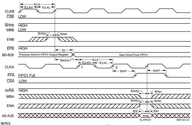
tskew is the minimum time between a rising CLKB edge and a rising CLKA edge for FFA to transition HIGH in the next CLKA cycle. If the time between the rising CLKB edge and rising CLKB edge is less than tskew1, then FFA may transition HIGH one CLKA cycle later than shown.
