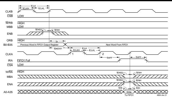
tskew is the minimum time between a rising CLKB edge and a rising CLKA edge for IRA to transition HIGH in the next CLKA cycle. If the time between the rising CLKB edge and rising CLKA edge is less than tskew1, then IRA may transition HIGH one CLKA cycle later than shown.
