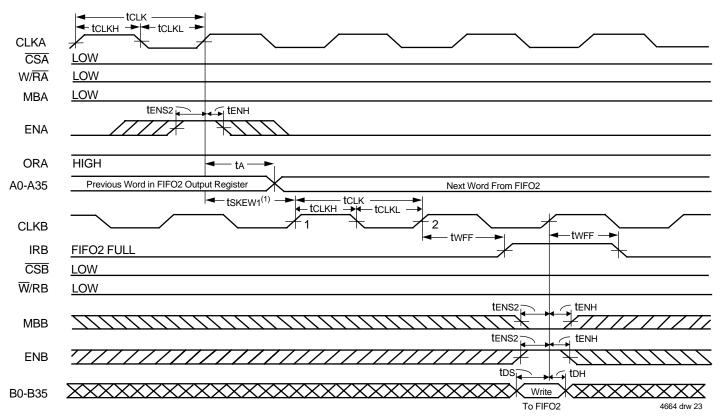
1. tskew1 is the minimum time between a rising CLKA edge and a rising CLKB edge for IRB to transition HIGH in the next CLKB cycle. If the time between the rising CLKA edge and rising CLKB edge is less than tskew1, then IRB may transition HIGH one CLKB cycle later than shown.
